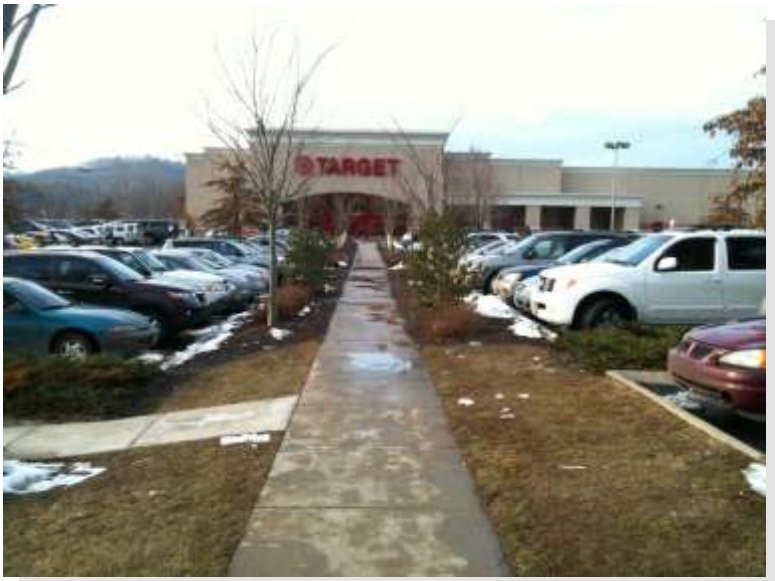
Cities can enact policies to require big box development to provide accommodations for pedestrians through parking lots. This example shows a center median route leading to the front door of the store. Such developments should have a route from the nearest street.
